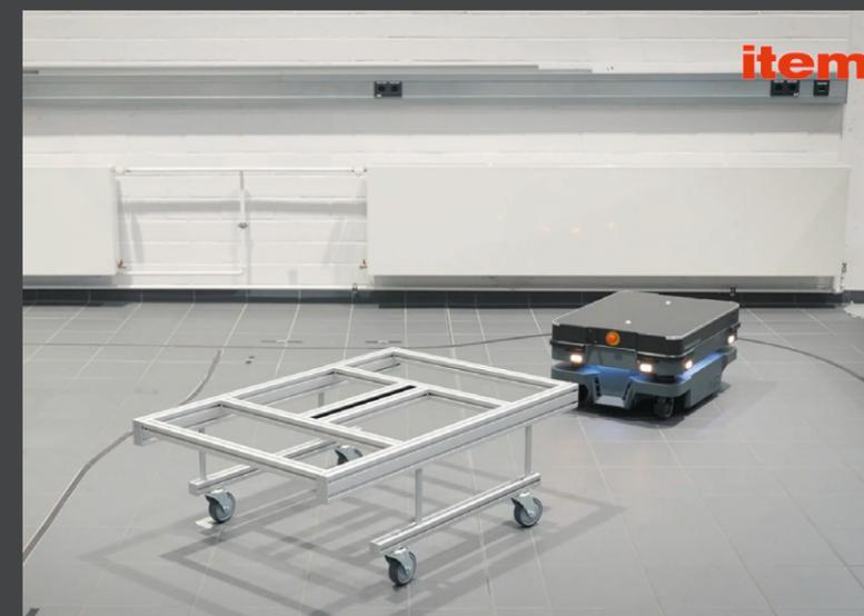
attachment can then be easily mounted on these Base Carts via the standard interface. As a result, the solution, consisting of a standardised base cart and individually configurable attachments, can be used for numerous applications.
