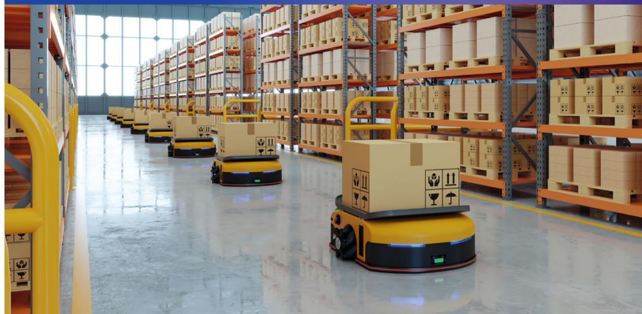
VDA 5050 was developed to solve this problem. It regulates the communication between the master control system and the individual vehicles. The standardization of the structure and content of the communication enables the smooth integration, control and optimization of different robot types as well as the smooth operation of hybrid fleets. This increases flexibility, efficiency and scalability.
